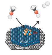
One metal or two? Adsorption and reaction studies on well-defined model systems are important to understand the complex surface processes on real catalysts. This fundamental study of the decomposition of methanol on metal clusters (see picture) results in syngas and/or carbon deposits on the particle surfaces depending on their composition.
